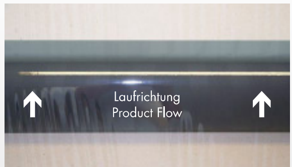
Flat spreading of sensitive foils on MITEX SoftSpreaders
