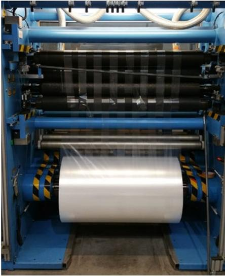
**Sandwich Roller and SoftSpreader in conjunction provide an optimum slitting result**
